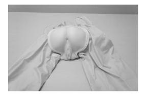
6. When fitting the simulator onto the dedicated mount, align the back of the simulator (black tube side) with the "hose connection side." In addition, when removing the simulator from the dedicated mount, disconnect the simulator from the groove located on top of the mount.
